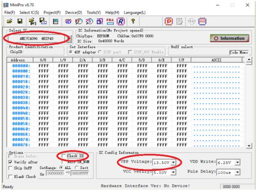
Set in MiniPro software EPROM 27C4096 or 27C240, select valid VPP Voltage and uncheck "Check ID" option!
